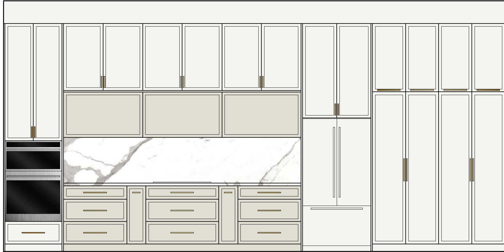
Typical Kitchen & Family Room Elevation Refer to millwork package for all model suite drawings
