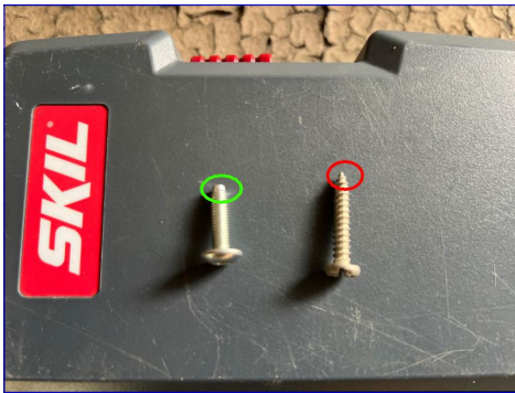
Correct vs. incorrect panel screws
