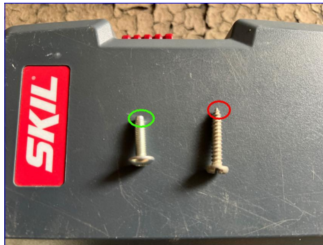
Correct vs. incorrect panel screws
