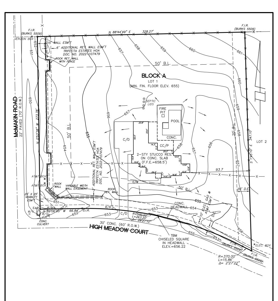
Basis of Bearing is the State Plane Coordinate System, Texas North Central Zone (4202), North American Datum of 1983, as determined from GPS observations.
