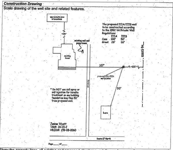
Show the property lines, all existing and proposed structures, existing and proposed sewage systems and water supplies, slope, and any topographic features which may impact the design of the well.
