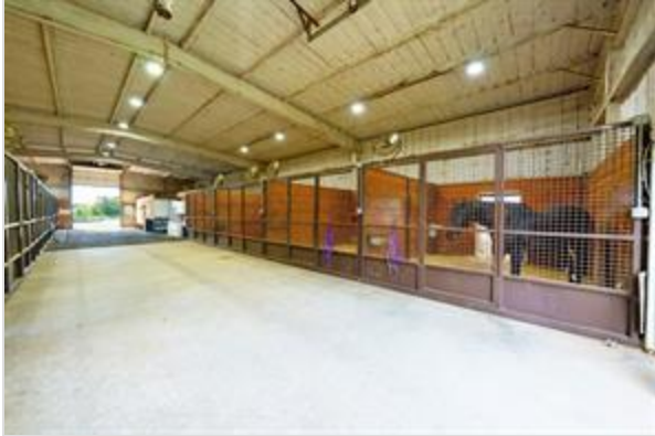
BARN INTERIOR...Extra View, Insulated, Welded Wire Stall Fronts, Stall Mats, Auto Waterers, W/D Hook-Ups In Tack Room, 6 Stalls Have Rear Doors To Runs
