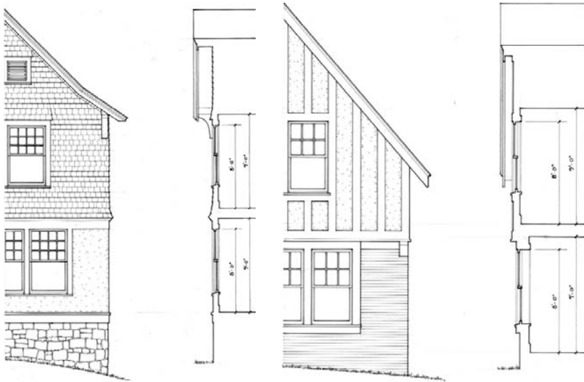
These partial section/ elevations illustrate typical profiles and exterior material combinations deemed suitable for Ramble homes.
