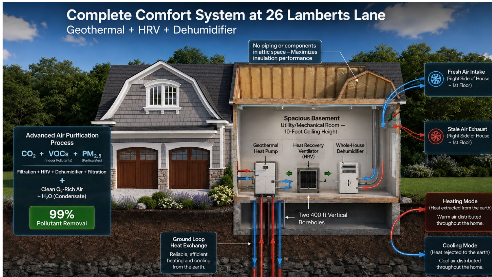
Complete comfort system diagram showing geothermal, HRV, and dehumidification concepts.
