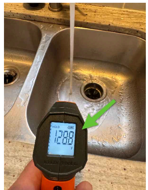
Typical hot water temperature
